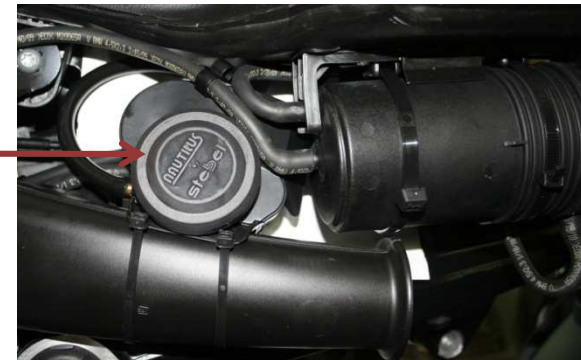
Horn mounted on air intake (Side view)
